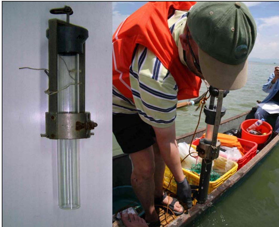
Figure 3. Miniature gravity corer (mini-corer) (left) and retrieving sample (right).
