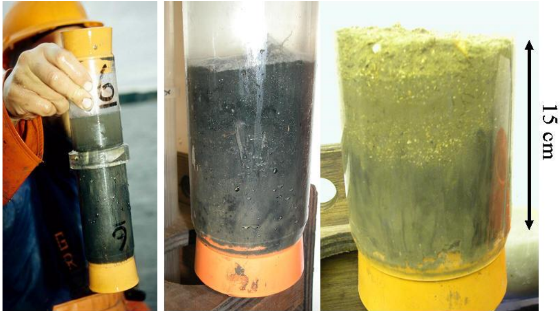
Figure 4. Sediment cores of the seabed taken underneath (middle photograph) and 40 m away (right photograph). The dark colour of the sediment in the middle photograph indicates heavy impact, and this was also smelly - there were no animals living in this sediment. The lighter colour of the core on the right indicates healthy sediments and there is a boundary at 7 cm - the surface layer above this is mixed by the animals living there.
