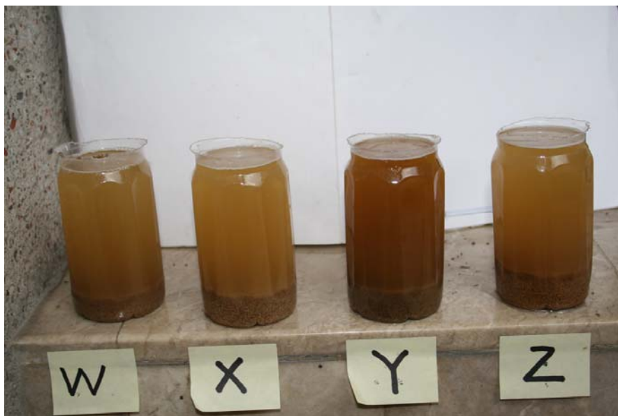
Simple experiment on feed stability using four of the most common aquaculture feeds used in the Philippines. This picture shows the dissolution of the feeds after 5 minutes.
